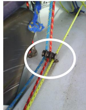
2. Bypass the existing up/downhaul cleat and take the rope through the extra pulley on the newly added triple block.
